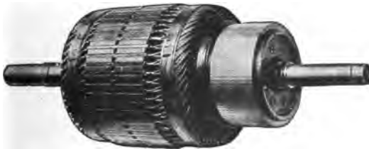
Completed Armature, Wound and Ready to Put Into Machine.
